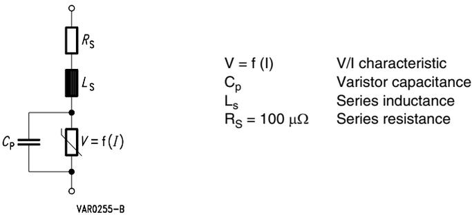
**Figure 16** Varistor model, basic structure
