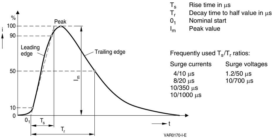
Figure 16 Waveform to IEC 60060 standard
