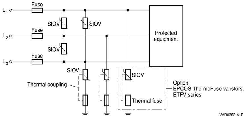
**Figure 4** Three-phase protection including line-to-ground protection
