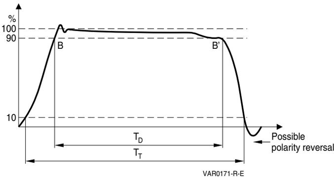
Figure 17 Waveform to IEC 60060 standard
