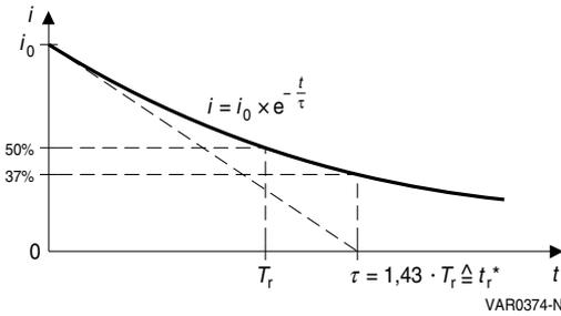
**Figure 9** Equivalent rectangular wave of an e-function
