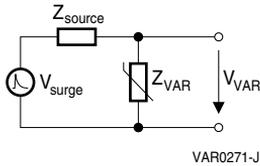
**Figure 1** Equivalent circuit in which  $Z_{source}$  symbolizes the voltage-independent source impedance
