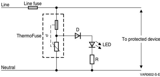
Figure 8 ETFV single-phase protection with working condition indicator
