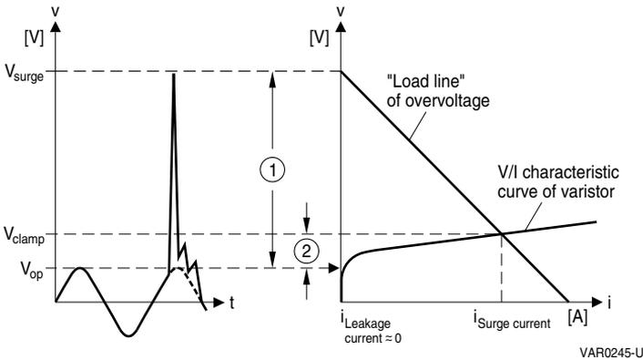
**Figure 2** Principle of overvoltage protection by varistors
