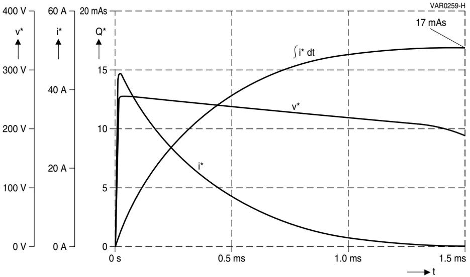
**Figure 20** PSpice simulation: voltage, current and  $\int i^* dt$  curves for the S10K95
